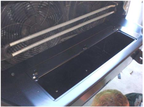
Figure 12: Bumper door, rear portion installed
