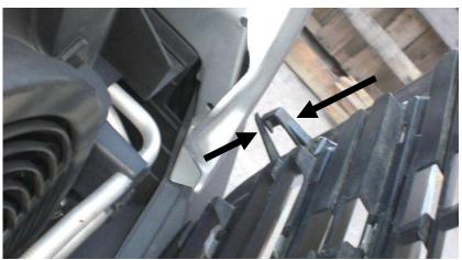
Figure 2: Grill retaining clips
