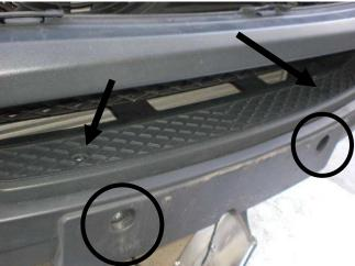
Plate cover (left) and plate cover removed (right) showing bumper cover fasteners
