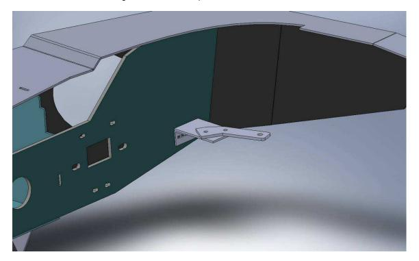
19. With the bumper hardware secured, bolt on the steel support brackets as shown in figure 9 below, using the supplied 1/2" hardware—the slotted hole aligns with the hole in the back surface of the bumper, and the smaller hole should be against the lower surface of the side of the frame—do not tighten these bolts down fully yet, you may have to move the bracket slightly
