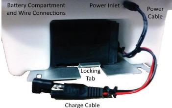
same sort of cable used to provide power on many laptop computers. We chose this style of cable for its ease of use. Simply plug it in with no worry of having it in the right way. <u>WARNING: Never plug in an AC Adapter that is rated for</u> output above 12 Volts and 5 Amps. Doing so could cause damage to your Laveo, and could cause a fire.
