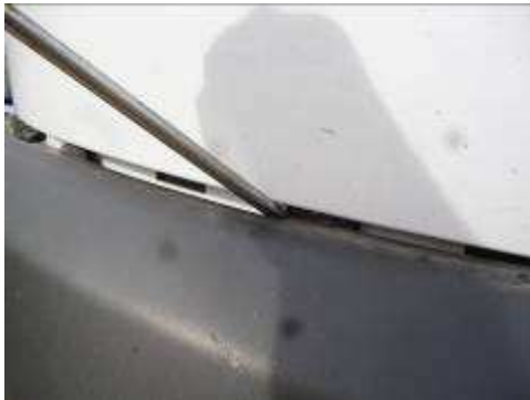
Figure 9: Prying Front Bumper from Grille
