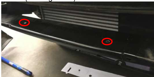
Figure 17: Holes Drilled Into Lower Sub-Frame
