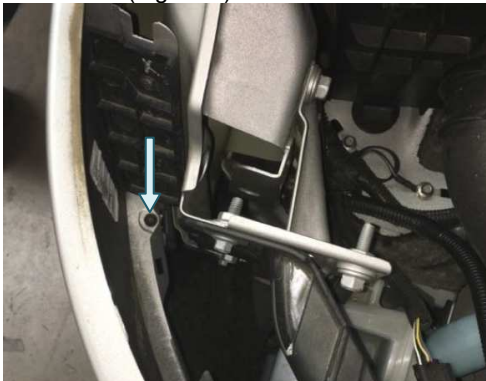
Figure 2: Bolts Underneath the Headlights
