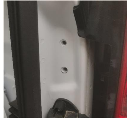
Figure 8: Factory Threaded Holes on Inside of Door Jam
