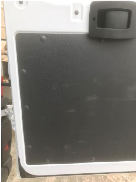
Figure 10: Remove Plastic Door Rivets
