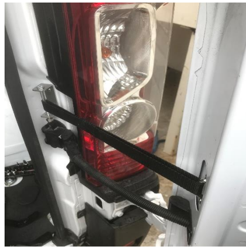
Figure 17: Completed Door Strap Installation
