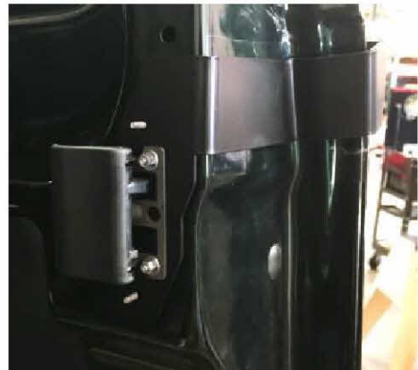
Figure 15: Upper Inner Passenger's Side Bracket Installed
