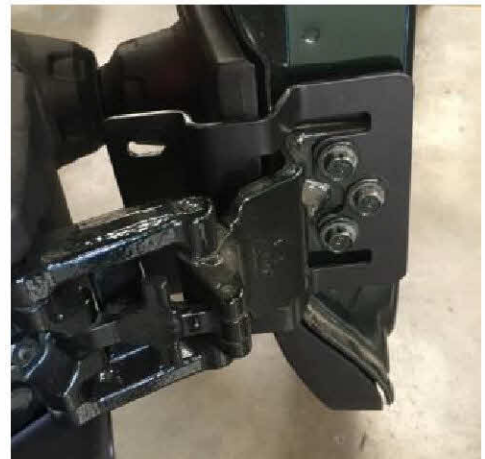
Figure 6: Inside View of Installed Lower Hinge Bracket
