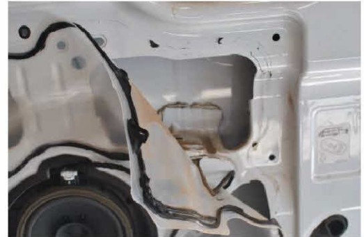
Figure 10: Inner Door Liner Peeled Back for Access
