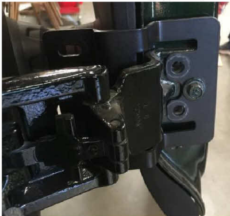
Figure 4: Hinge Placed Back into Position
