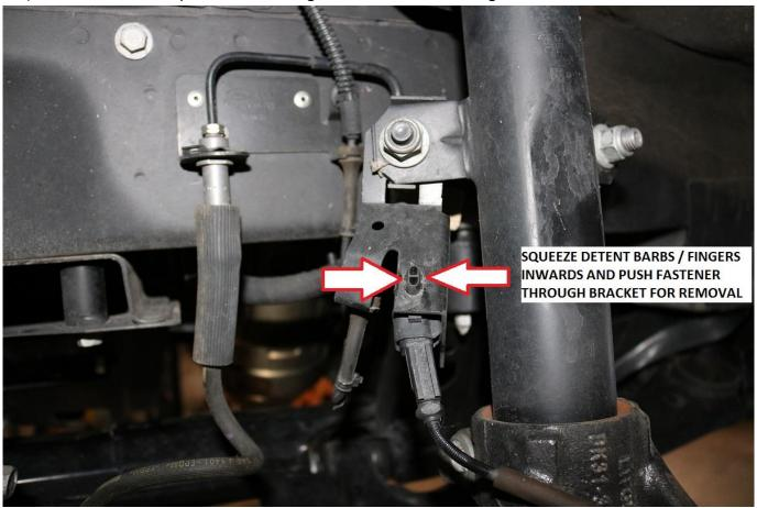
13) Completely remove the wheel speed sensor wiring from the strut. Separate the wheel speed sensor from the chassis harness. See image below for reference.
