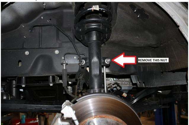
12) Remove the wheel speed sensor wiring from the strut. See image below for reference.
