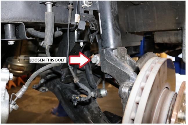
16) Loosen the front lower control arm bolt. Use a 21mm socket / wrench. See image below for reference.
