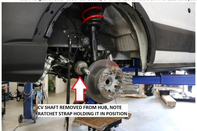
21) With the CV free from the hub, support the steering knuckle with a transmission or floor jack and remove the 18mm lower strut bolt. Remove the steering knuckle from the strut and set it aside.
