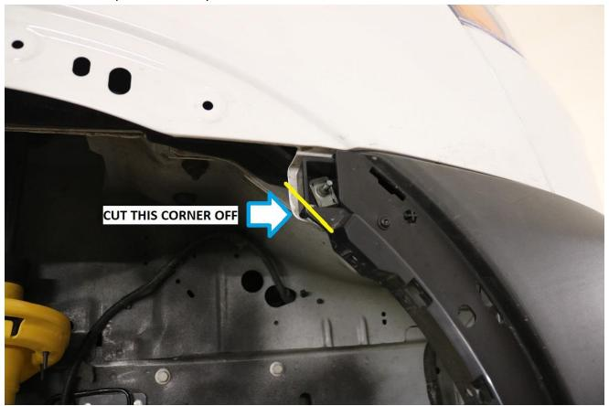
46) Lastly, the front bottom corner of the plastic front bumper fascia needs to be trimmed slightly for tire clearance.
