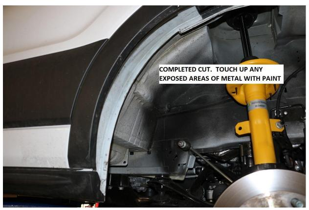
45) Towards the front of the wheel opening, locate the inner M6 bolt securing the front bumper fascia to the vehicle. There is a small flange that needs the corner cut off. Note, the outer fender trim piece is removed in this photo for clarity.
