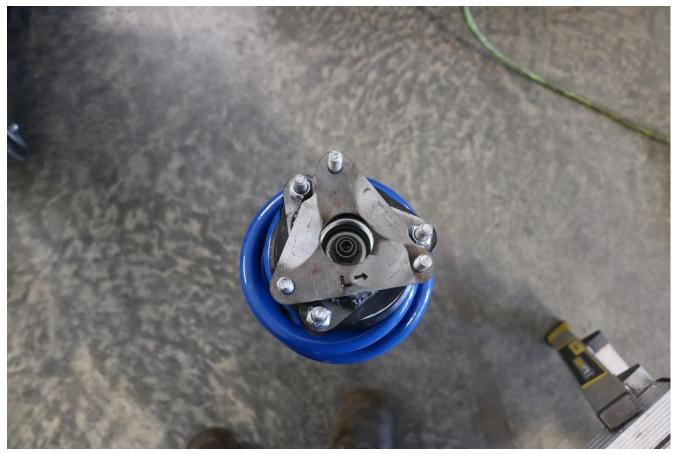
29) Use a 4-1/2" angle grinder or similar cutting tool to cut the studs flush or close to flush with the top of the installed stover nuts. Be careful to not cut the spacer or nick the powder coat while cutting.
