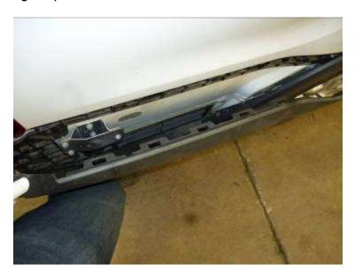
18. With the torx bolts removed carefully pull the upper part of the side panel away from the vehicle. It is just clipped in and should slide out.
