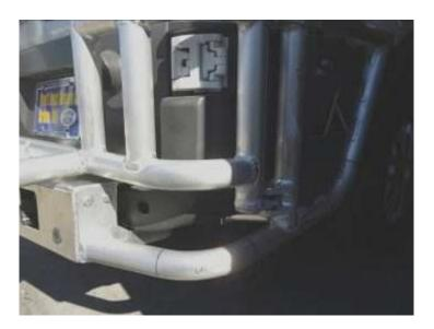
28. Loosely install the (3) 3/8" by 1.5" stainless bolts to hold the swing arm structure to the bumper. Do not tighten these yet.
