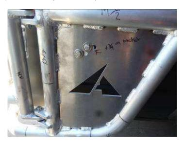
29. With the swing arm structure loosely held to the bumper you can line up the hole in the logo plate with the swing arm support that was installed behind the side panel of the vehicle. Use the 3/8" by 1.5" stainless bolt with locktite and tighten the swing arm structure to the swing arm support.
