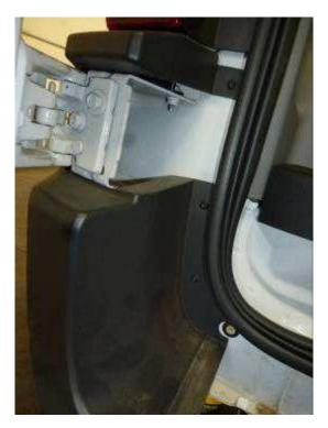
12. Remove the 3 torx bolts holding each plastic end cap to the body.
