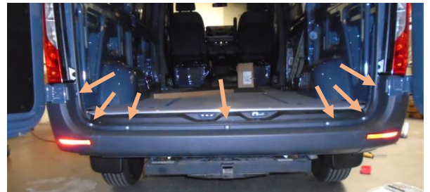
Figure 2: Torx Bolts on the Rear Bumper
