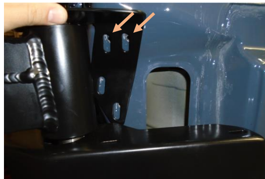
Figure 11: Drilling for Axle Support Bracket
