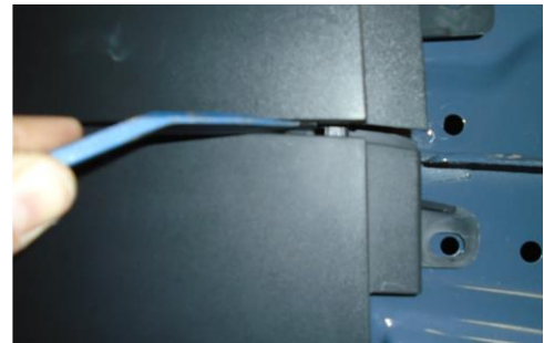
Figure 7: Removing Small Plastic Panel from Rear Bumper
