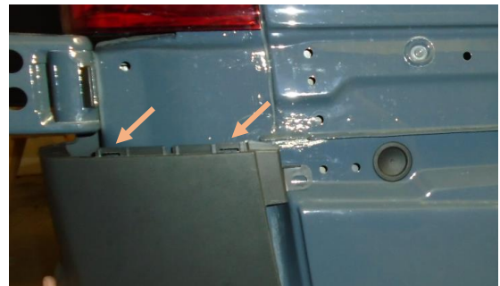
Figure 8: Small Plastic Panel Removed
