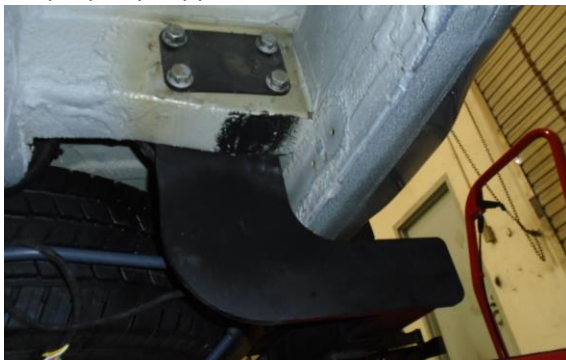
Figure 1: Four (4) of the Hitch Mounting Bolts
