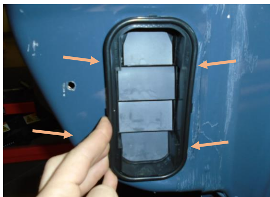
Figure 9: Air Pressure Relief Insert Removal
