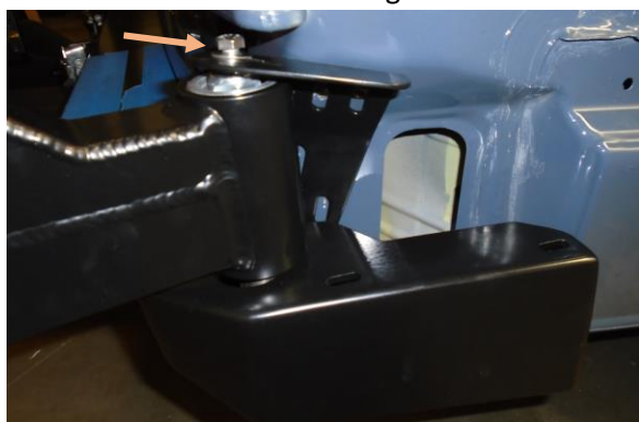
Figure 10: Pre-Mounting Axle Support Brackets
