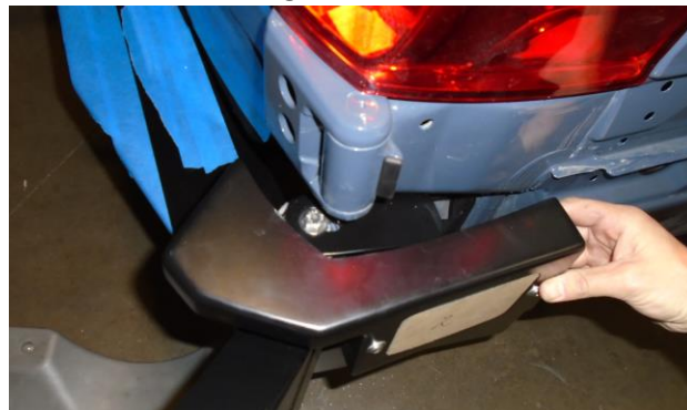
Figure 13: Installation of the Trim Assembly
