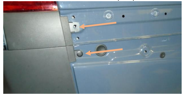
Figure 6: Plastic Rivets Underneath the Side Panel
