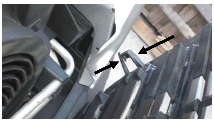
Figure 2: Grill retaining clips
