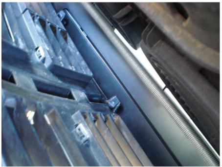
Figure 13: Stock grill installed on Aluminess door tabs
