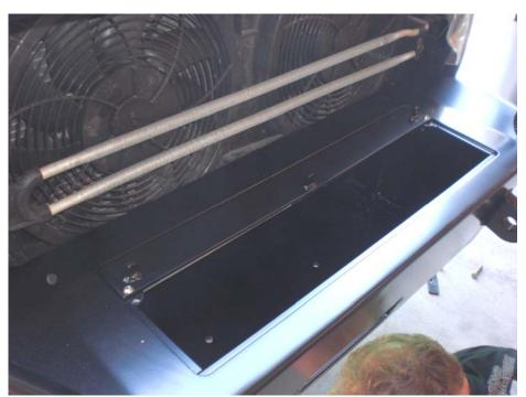
Figure 12: Bumper door, rear portion installed
