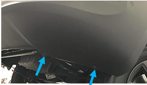
Figure 8: Plastic Rivets on Underside of Bumper
