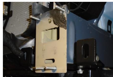
Figure 16: M8 Bolts Installed
