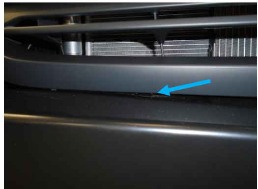
Figure 30: Grille Tabs Installed
