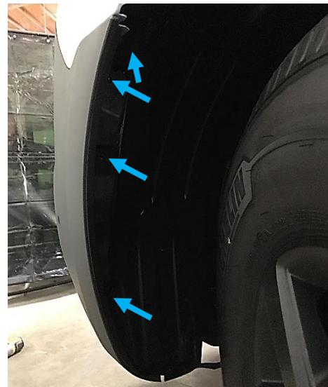
Figure 7: Plastic Rivets on the Inside of the Wheel Well
