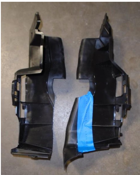
Figure 19: Plastic Shrouds Cut (left) and Uncut (right)
