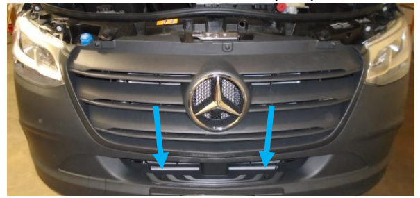
Figure 5: Plastic Cap Location
