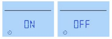
The time switch is only enabled once until it is disabled (turned off) or powered down. If the timer switch is programmed and enabled, the time switch icon is displayed in the status line (2). The timing icon flashes if the time switch is enabled and activated.
