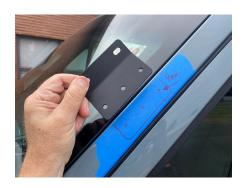
**Step 8.** Install upper bracket on snorkel using the two M6 bolts. Install snorkel onto Sprinter with provided allen head bolts and washers, snug but not tight. Place blue painters tape on the "A" pillar where the bracket lands. Using your marker, mark where the bracket will sit on the tape.
