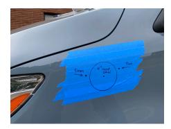
**Step 4.** Drill the 2 9mm holes using the provided 9mm drill bit.
