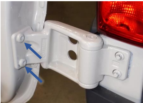
Figure 4: Inside View of Lower Hinge
