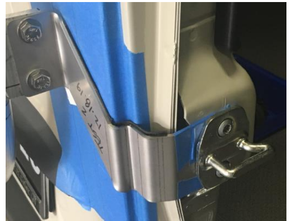
Figure 7: Installed Latch Pin Bracket
