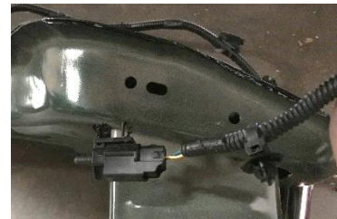
Figure 17: Temperature Sensor Removed
