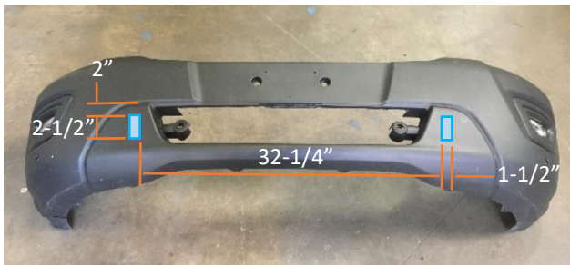
Figure 34: Tow Hook Cut Location
