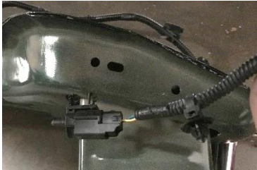
Figure 18: Temperature Sensor Removed
