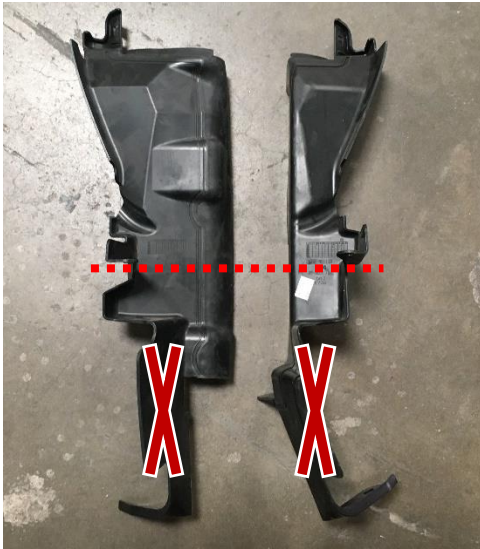
Figure 17: Radiator Air Deflector with Cut Line Shown
