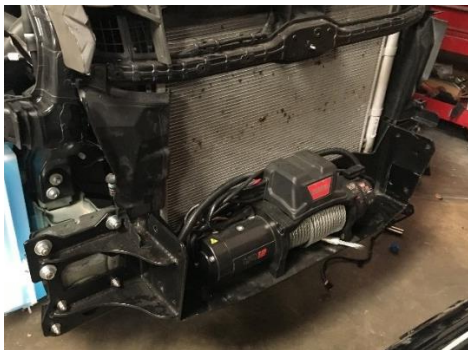
Figure 29: Winch Installed onto Winch Plate
