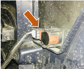
Figure 14: Parking Sensors from Backside of Bumper
