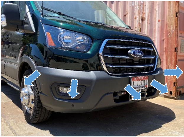
Figure 12: Factory Bumper Removal
