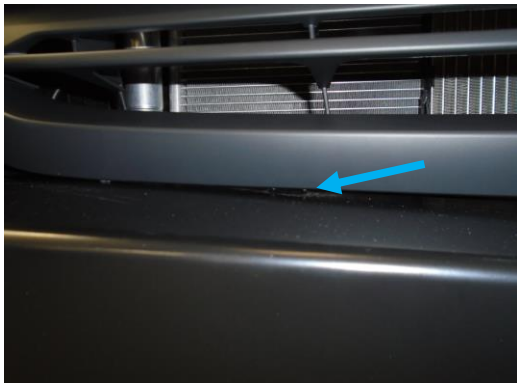
Figure 29: Grille Tabs Installed
