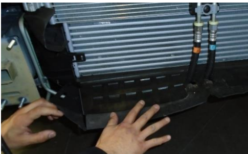
Figure 15: Air Flow Skirt Pressed Down
