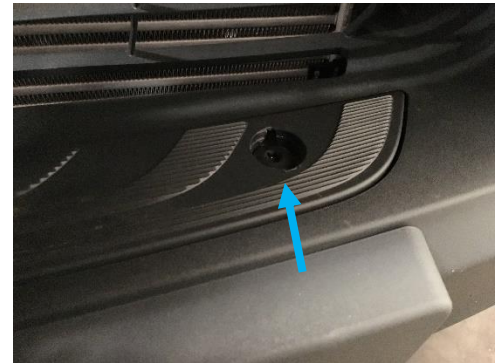
Figure 6: Front Bumper Step with Plastic Cap Removed
