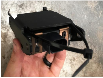
Figure 23: Feed a Zip Tie Between the Sensor and Sensor Carriage (Behind Sensor)
