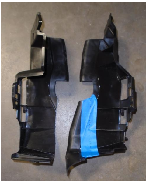
Figure 19: Plastic Shrouds Cut (left) and Uncut (right)
