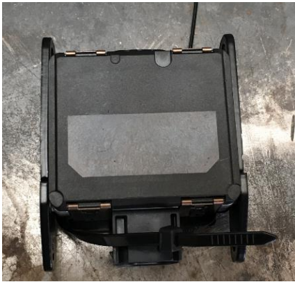
Figure 24: Pull the Zip Tie(s) Around the Front of the Sensor Connection
