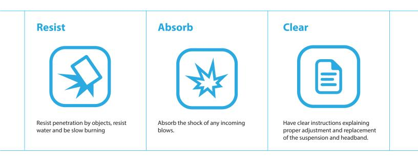
Hard hats must have a hard outer shell and a shock-absorbing lining that incorporates a headband and straps that suspend the shell from 1 to 1 1/4 inches (2.54 cm to 3.18 cm) away from the head. This type of design provides shock absorption during an impact and ventilation during normal wear.
