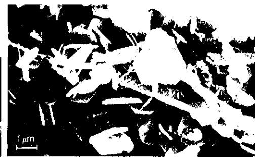
□ Scanning-electron micrograph showing biofilm surrounding a corrosion pit. Enlargement, inside the pit, shows crystals of metal corrosion product, probably iron sulfide (planar objects), interspersed with bacteria (cylindrical objects).
