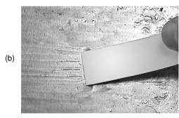
(b) Draw moistened pad across a line on the test surface approximately 2 inches (5.1 cm) in length. Reverse direction, sampling same area a second time.
