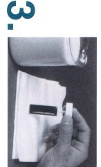
Allow excess fluid to drain from paddle. To avoid outside contamination, be careful not to touch the paddle to any other surface before replacing in tube.
