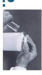
Immerse the paddle into the fluid sample for 2–3 seconds so that both surfaces are covered.
