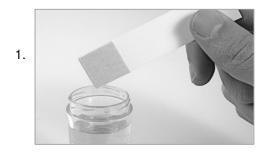
Dip pad end of strip into sample for 5-10 seconds. For non-aqueous liquids, the pad must be pre-wet with sterile water.
