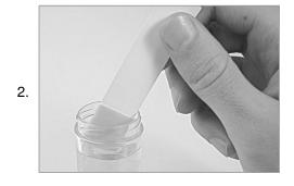
Remove strip from sample and shake off excess liquid.
