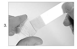
Open transparent pouch and insert test strip.
