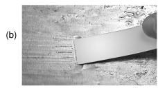
(b) Draw moistened pad across a line on the test surface approximately 2 inches (5.1 cm) in length. Reverse direction, sampling same area a second time.
