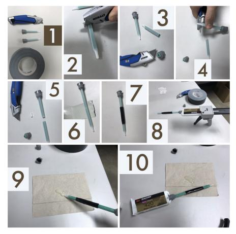
**Steps 8, 9, 10:** The mixing nozzle can then be affixed to the adhesive cartridge and successfully mix and dispense the adhesive as normal. The longer mixing nozzle will then properly mix more sensitive adhesives.
