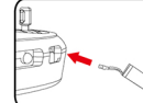
B. Connect the lithium battery with the charging interface on the remote controller to charge up.
