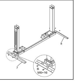
STEP 3 Assemble feet (11) to legs using M6x16 bolts (B), making sure both feet are facing forward, and tighten with the Allen wrench (D). Snap plastic covers (10) onto the short ends of the feet. B D
