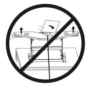
Leave enough slack in cable to allow for full range of vertical motion (15" / 38 cm). Failure to heed this warning may result in property damage and or personal injury.
