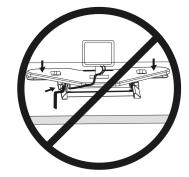
To avoid the potential to pinch cables it is important to follow the cable routing instructions in this manual.
