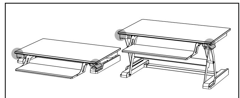
**Step 1**: Squeeze the handle on the underside to raise the unit. Lift using both handles.
