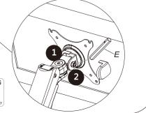
A If the monitor cannot stop at any height, pls use 5x5 allen key(G)to adjust the screw on the arm.
