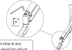
To adjust the swivel function by 5x5 allen key(G) on position 1
