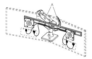
2. Route power and monitor cables through the flexible cable clips on the M8.1's upper link (B).
