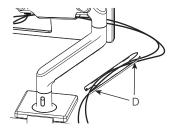
5. Lift the cover and cables up to the lower link, making sure that the cover sits flush with the surface of the arm.
