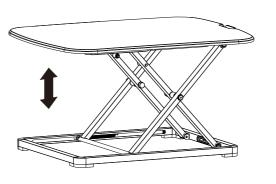
To lower the desk, use your thumb to flip the switch and then release. The weight of the desk will automatically lower it to the next level. The device will give a voice confirmation when the desk enters the next height level and will auto matically lock in place.
