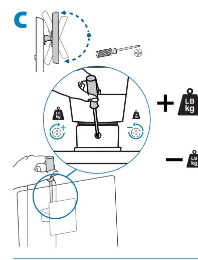
Increase Lift Strength If the mounted weight is too heavy or this product does not stay up when raised, then you'll need to increase Lift Strength:
