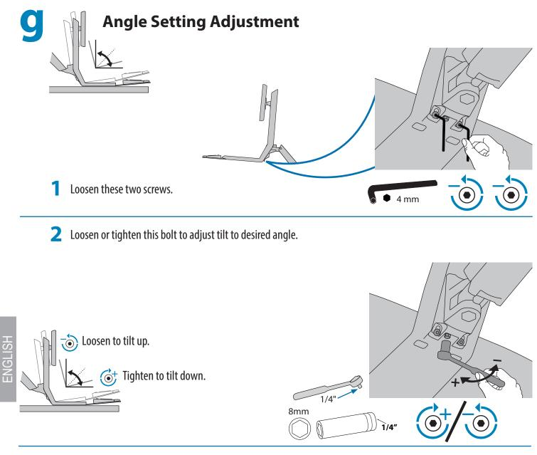
**3** After desired tilt is achieved, retighten these two screws to secure.
