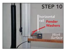
**Step 10:** Lift the Work Surface up and align the holes in the Horizontal Rail with the (2) 1/4-20 x 3.50 Hex Head Bolts{B}. Push the Work Surface onto the Hex Head Bolts until the threads of the bolts come through the Horizontal Rail.
