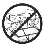
Leave enough slack in cable to allow for full range of vertical motion (15" / 38 cm).
