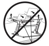
Leave enough slack in cable to allow for full range of vertical motion (15" / 38 cm).
