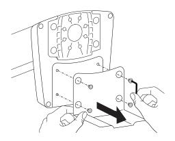
Position arm with attached grommet plate over grommet hole (make sure bolt is centered in hole). Thread grommet bracket and wing nut onto bolt and tighten.
