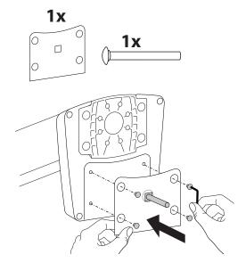
Remove clamp plate screws with 4mm hex wrench. Retain screws.
