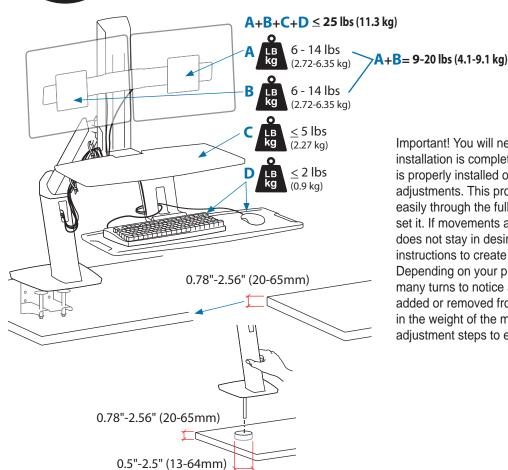
Important! You will need to adjust this product after installation is complete. Make sure all your equipment is properly installed on the product before attempting adjustments. This product should move smoothly and easily through the full range of motion and stay where you set it. If movements are too easy or difficult or if product does not stay in desired positions, follow the adjustment
