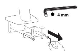
Insert provided bolt into provided grommet plate. Attach grommet plate with 4 mm hex wrench and screws removed in step b.
