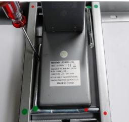
With the green-dotted end all way into the hole, use your hand to push lever **TOWARDS** the lifting column. You should feel some pressure while pushing the lever down. Once the lever is flush with the beam, use a tool like a flat-head screwdriver to push it all the way down until it touches the surface where the beam rests. If no pressure is felt while pushing the lever down, check whether the top support bracket is installed and secured properly.
