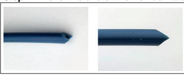
Place the end of the Bowden tube on a flat surface, and use a sharp knife to cut bevels on the end, making a 90-degree peak.
