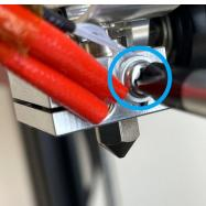
• Place the heater cartridge and thermistor into the heater
