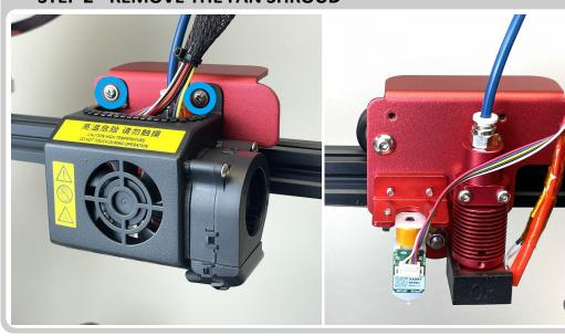
• Remove the two screws holding the fan shroud.
