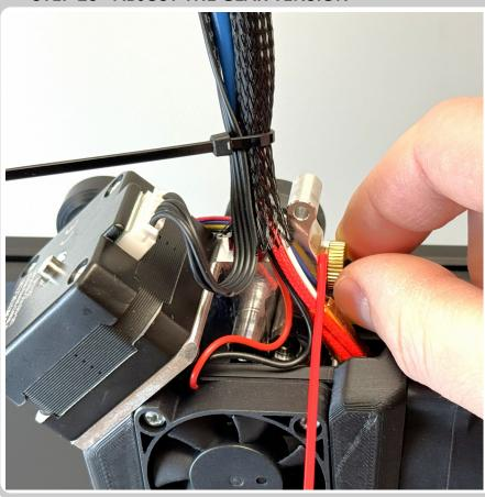
• Adjust the gear tension by rotating the brass knob.
