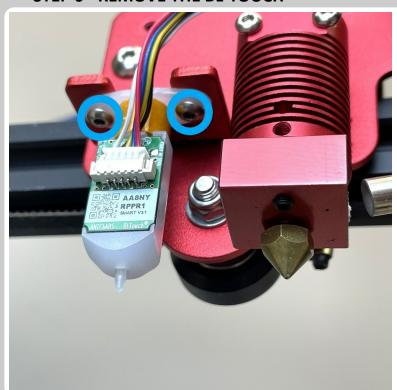
• Remove the two screws holding the BL-Touch. (2.0mm Allen wrench)
