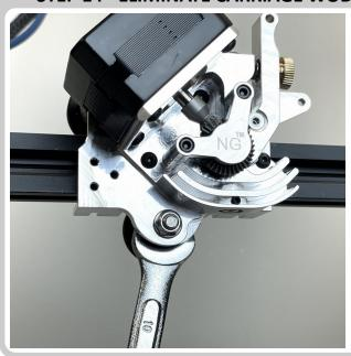
• Adjust the bottom V-Roller wheel position by rotating the eccentric nut to eliminate any carriage wobble.
