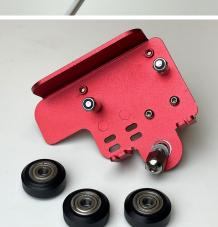
• Remove the three V-Roller wheels. (3.0mm Allen wrench and 8mm spanner wrench)
