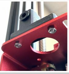
• Attach the 3D printed PTFE Bracket beside the Filament Runout Sensor using the provided M3 screws and M3 nuts.
