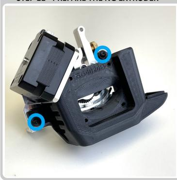
• Detach the NG fan shroud from the extruder by removing the two screws that secure it in place.
