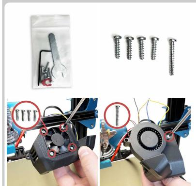
• Install the hotend cooling fan onto the fan shroud using the four smaller self-tapping screws
