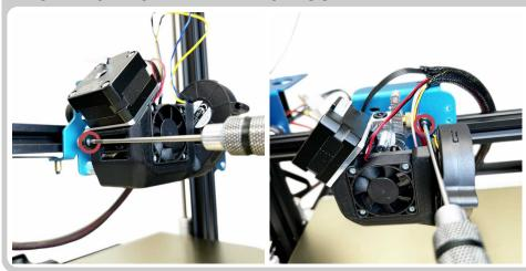
• Install the fan shroud back on to the NG Extruder
