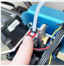
• Using the provided M3 screw and nuts, attach the 3D printed Guide Tube Bracket in the spot where the printer's original Bowden Extruder used to be
