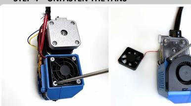
• Detach the hotend fan from the stock fan shroud by unscrewing the 4 screws
