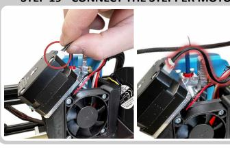
• Connect on NG Extension cable to the stepper motor
