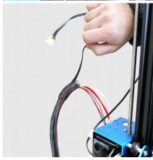
The long stepper motor extension cable going to the print head needs to be removed because it will be replaced with the NG Extension cable in step 8
