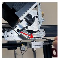
• Insert the hotend assembly into the extruder
