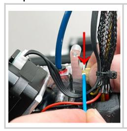
Adjust the gear tension by rotating the brass knob
