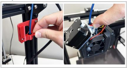
The printers original Bowden tube will be reused to help guide filament from the spool into the Extruder
