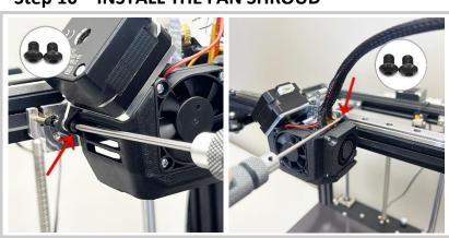
Install the assembled fan shroud back on the extruder
