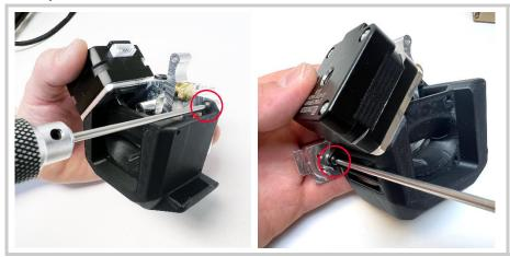
Detach the fan shroud from the extruder assembly by removing the two screws using a 2mm Allen wrench
