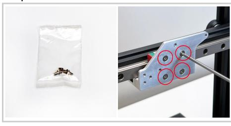
Attach the Linear Rail Adaptation Plate to your linear rail's carriage block using the provided M3 x .5 x 6mm Flat Head Cap Screws
