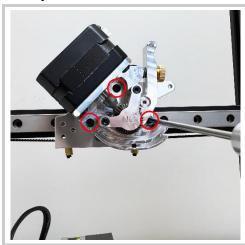
Re-attach the NG Extruder Main Body to the Adaptation Plate using the three M3 screws using a 2mm Allen wrench
