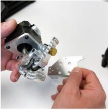
Detach the Extruder Main Body from the Adaptation Plate in the back by removing the three screws using a 2mm Allen wrench
