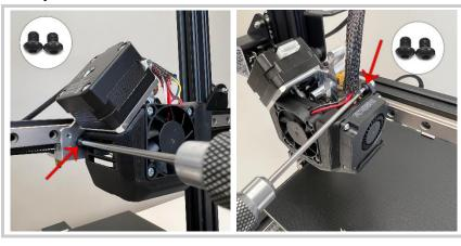
Install the assembled fan shroud back onto the extruder
