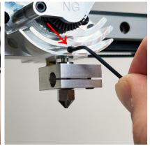
• Attach the hotend assembly to the extruder
