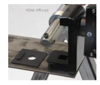
Step 6) Install the stainless steel  $\frac{1}{2}$ " flat washer,  $\frac{1}{2}$ " lock washer, and  $\frac{1}{2}$ " nut on both mounting bolts. Only install  $\frac{1}{2}$ " nuts with a few turns. *Important:* The  $\frac{1}{2}$ " nuts must be left loose so the load brackets can be lifted up off the mounting surface to install interlocking security brackets in Step 7.
