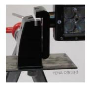
Step 8) Grab the threads of the carriage bolt and turn back and forth to ensure the square shank of the blot is still in the square hole of the load bracket. After checking bolt is in place apply a slight downward force on  $\frac{1}{2}$ " nut to keep the bolt in place as the nut is screwed on. Tighten until finger tight and then repeat on second mounting bolt at the opposite end of the light bar.
