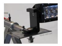
Step 7) Lift up the light bar to slide the security bracket underneath the load bracket. Align the raised tab facing up (Step 5) with the slot in the base of the security bracket. Then lower light bar to couple both brackets together. Repeat process with the other bracket set at the opposite end of the light bar before tightening either of the two  $\frac{1}{2}$ " nuts.
