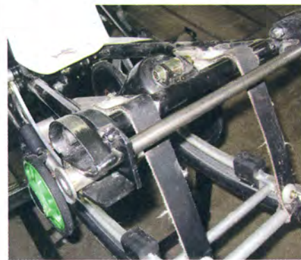
There is some slack in these limiter straps, which is how they should be when installed in a sled's chassis.
