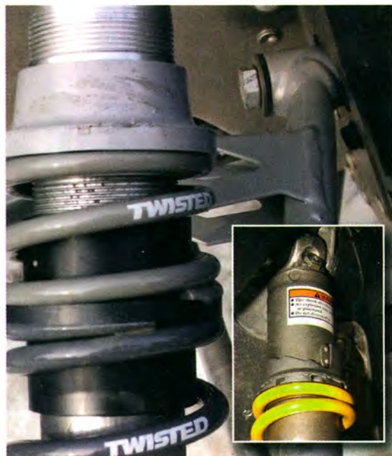
Ski-and center-shock springs usually use a cam (inset) or threaded collar to set spring preload.
