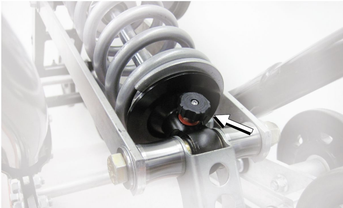
Damping adjuster used for ride quality.
