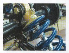
The black, crescent-shaped piece that's fastened with the same bolts that fasten the shock (top) and link rods (bottom) is the special linkage that changed the suspension's motion ratio.
