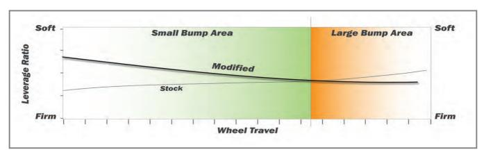
Coil over spring shocks may need a new single rate spring, depending on rider weight. It seems to work best with riders in the 200-250 pound range. Lighter riders will find the best performance with a lighter straight rate spring, where heavier riders will be best suited with a heavier straight rate spring. Further ride improvements can also be made by revalving the shocks, and making other modifications such as adding adjustable reservoirs.
