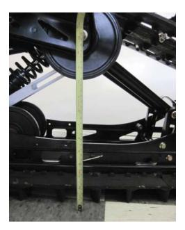
Place rider and gear on vehicle and re-measure. This should be 2/3 the distance as the previous measurement without rider. Adjust preload as necessary to achieve this.
