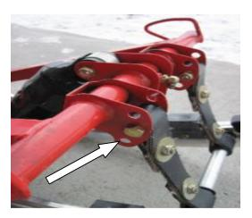
The front arm should be mounted in the upper hole.
