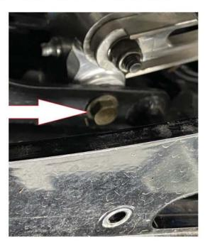
The cam will need to be levered into position in order to install the lower mounting bolt.
