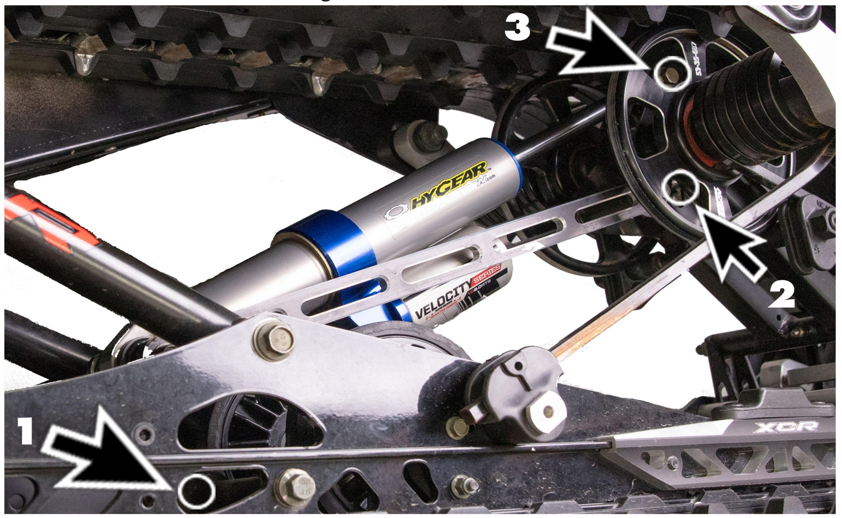
To remove the OEM linkage and shock assembly start by removing mounting bolts in the order of: 1,2,3 as shown.
