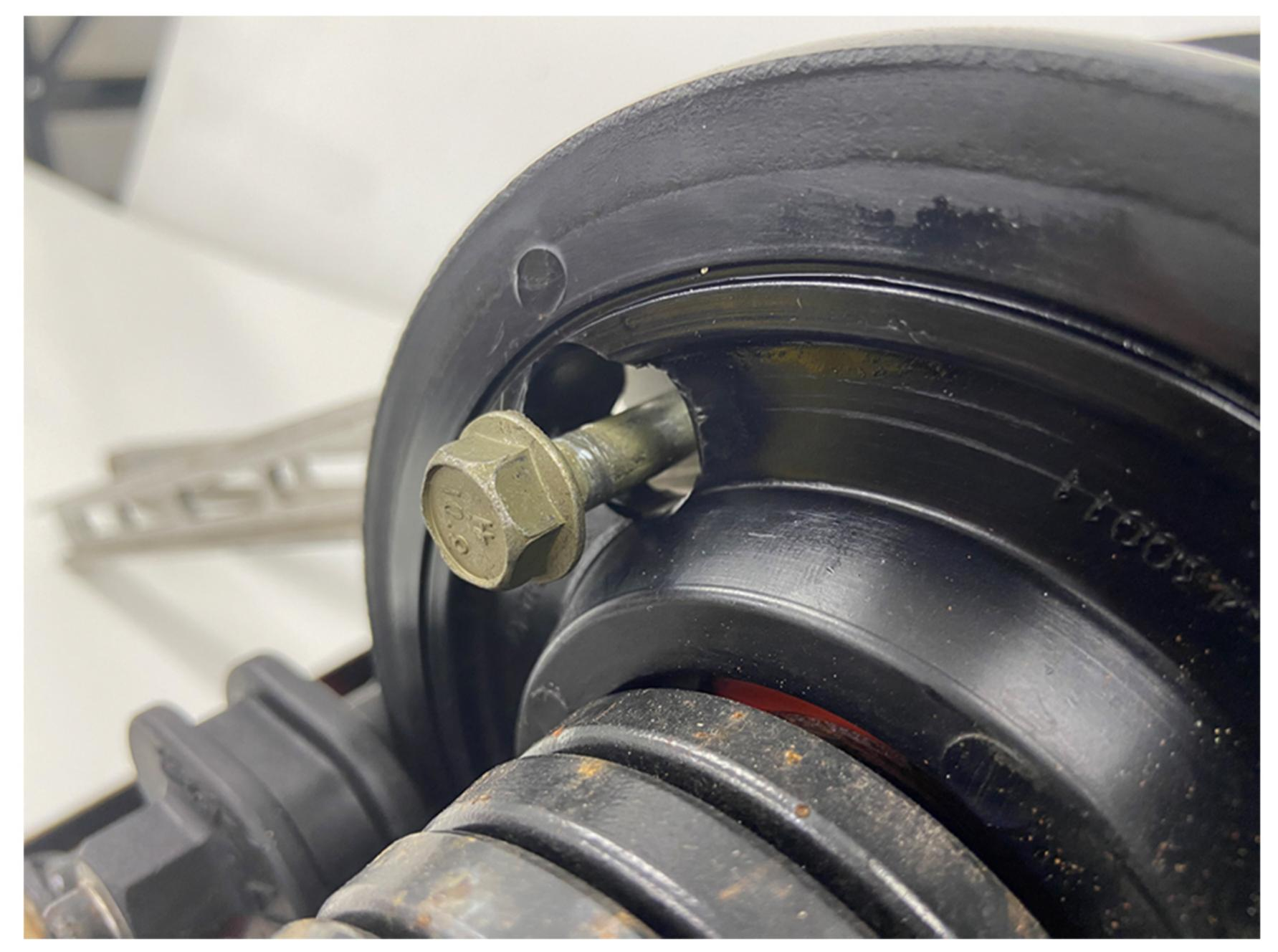
The rear arm idler wheels have access holes to remove the rear shock mount and link rod pivot bolts.
