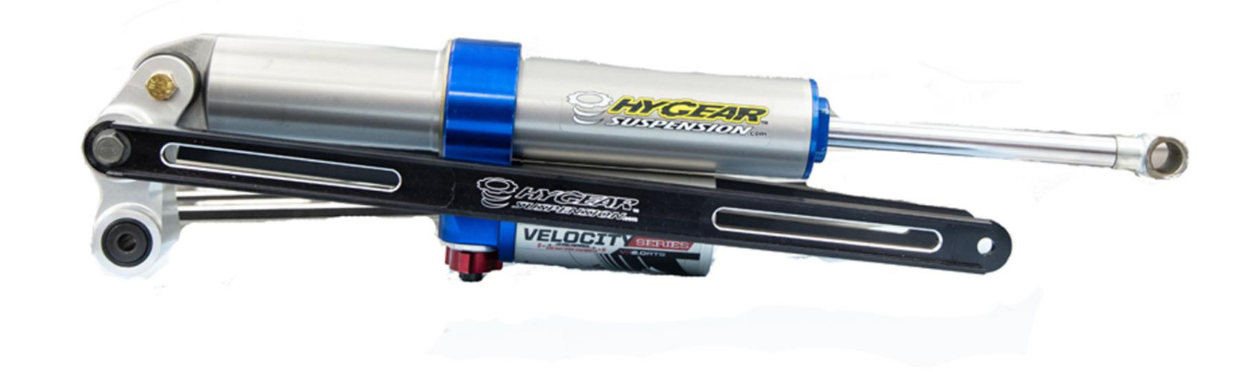
Note the shock mounting orientation and the direction of logo placement on the link rods for proper assembly before installing back into the suspension.
