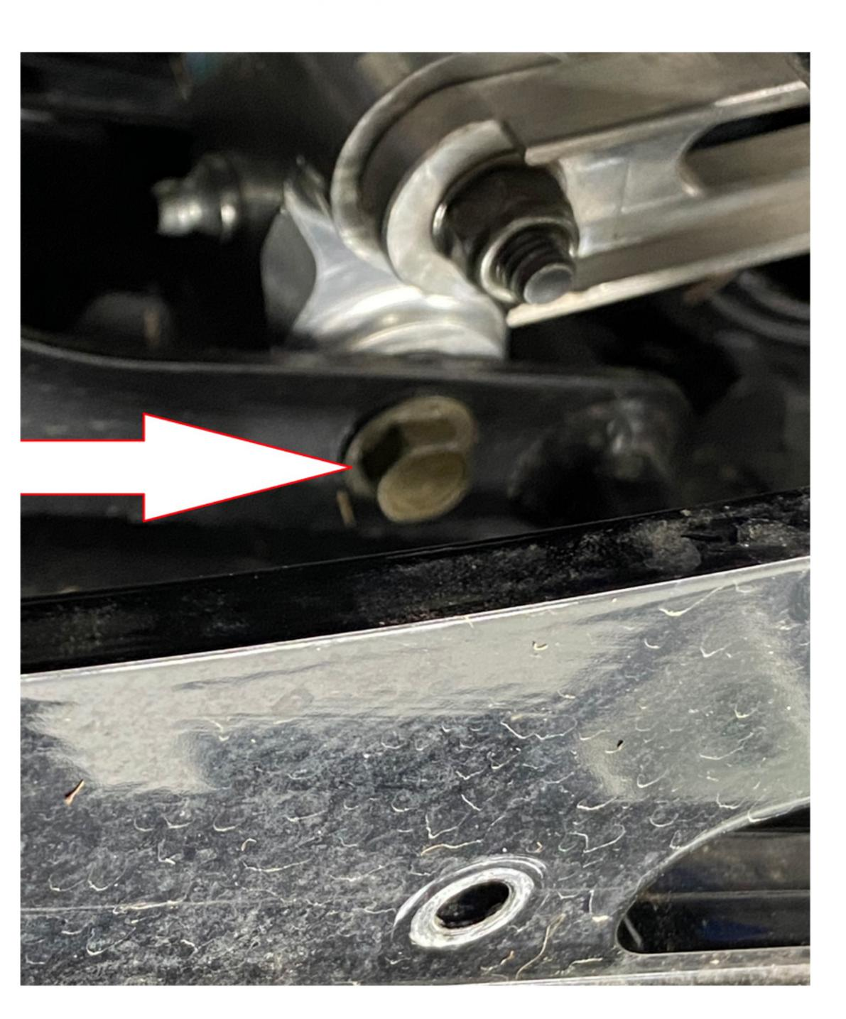
The cam will need to be levered into position in order to install the lower mounting bolt.
