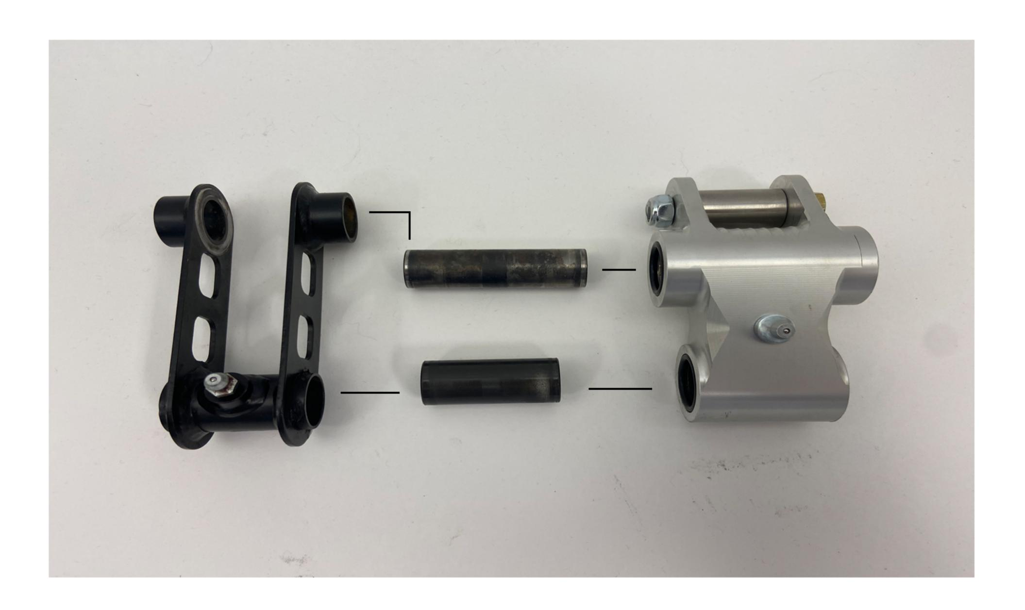
Reuse the two mounting pins from the OEM link. Install both into the cam and ensure the O-ring seals are properly seated.
