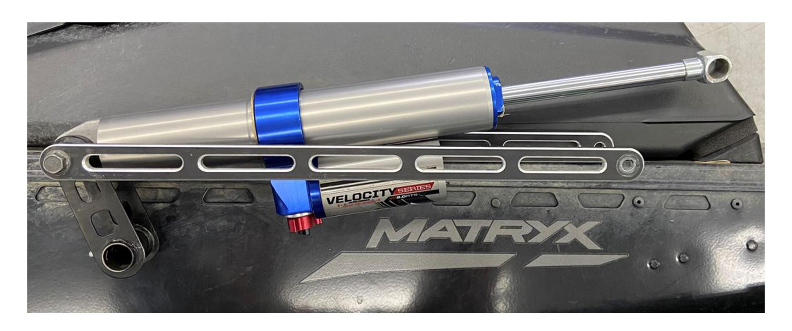
Remove the OEM shock and link rod assembly from the rear suspension.
