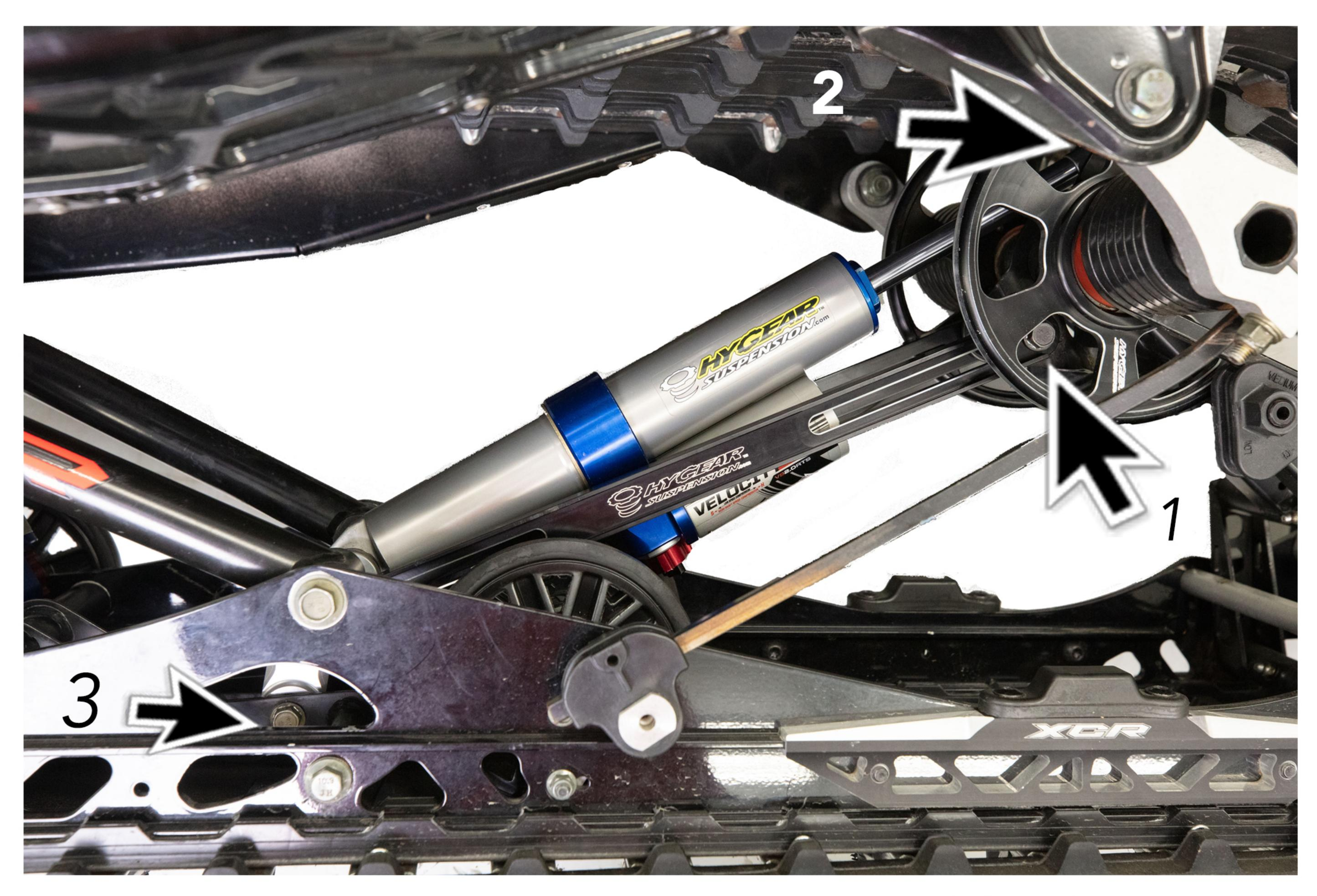
Start by installing mounting bolts in the order of: 1, 2, 3 as shown.
